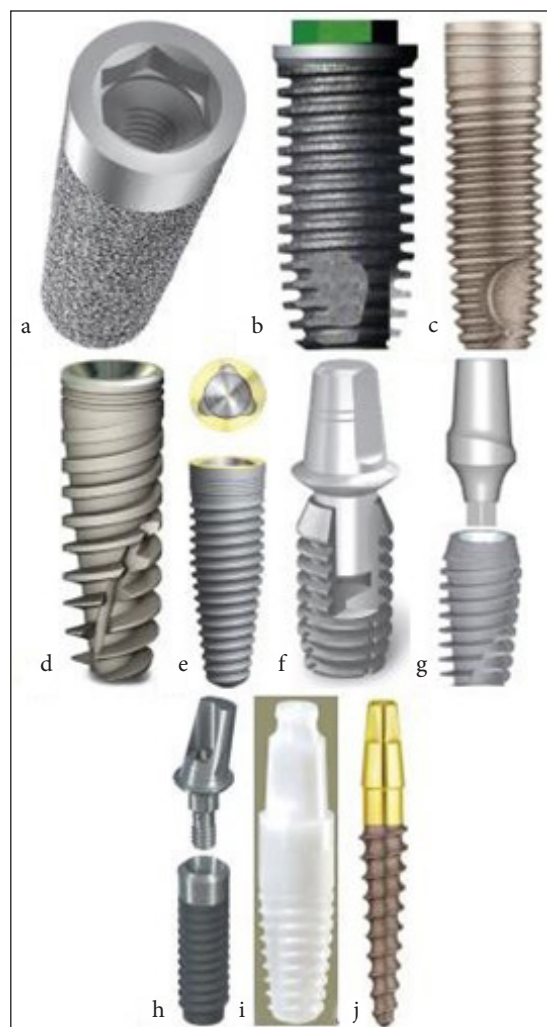
Figure 1: Different Implant Design. (a) - Non-threaded implant of Endopore system with hexagonal internal connection. (b) - Threaded implant with square threads and hexagonal external connection. (c) - Parallel body design with self-tapping thread design from Alpha Bio. (d) - Tapered body with variable thread design. (e) - Tapered implant from Nobel Biocare with triangular internal connection. (f) - Tapered internal connection implant. (g) - Taper internal connection. (h) - Soft tissue-level single-stage implant from Straumann. (i) - White zirconium implant. (j) - One-piece implant
