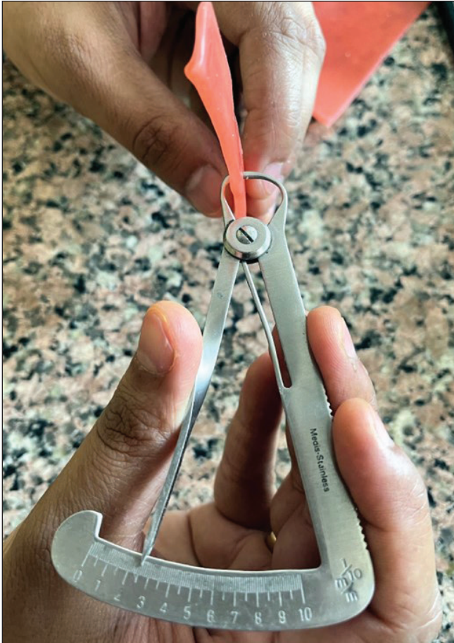
Figure 6: Spacer thickness verification using Dental Gauge Wax Caliper.
